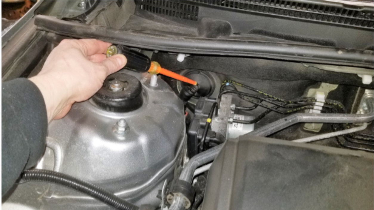
Figure 4 As pointed to by the individual with the screwdriver, the hole that allows wires through the engine bay back to the cab, or the “firewall”, is located on the side at which the fuse box is located in the cabin, usually on the driver’s side of the car. (Cesar, 2020)
