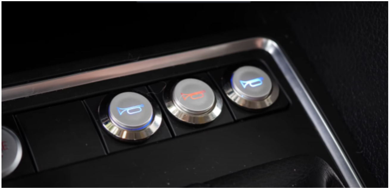
Figure 1 The buttons shown in this image demonstrate their placement in the car, which is just above the gear shifter stick that is located right below the radio. This location is good especially for drivers who tend to overuse the 110 dB normal car horn where they would have to reach to this location to use it. (Rober, 2017)
